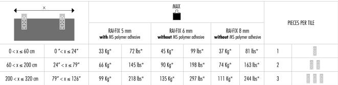
Conservatively, in the tables it has been considered halved loads for 6 and 8 mm hooks and equal to 25% loads for 5 mm hooks compared to the maximum potential measured by the laboratory.
